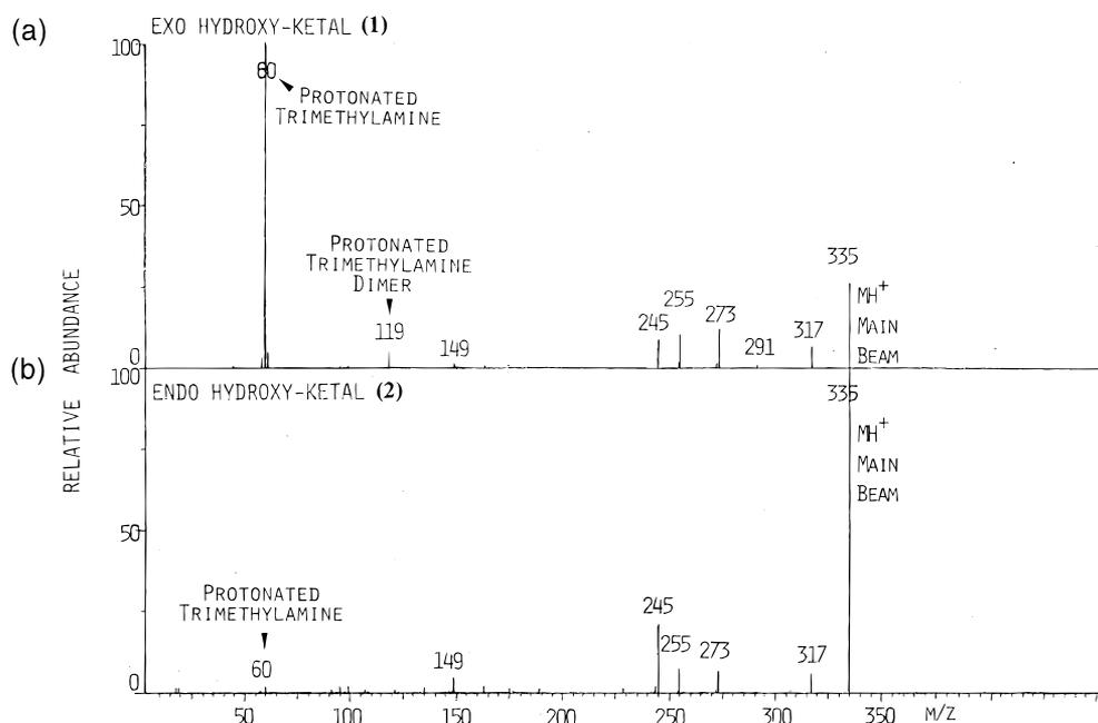
**Figure 3.** Collisionally activated reaction mass spectra of MH<sup>+</sup> (*m/z* 335) from (a) *exo* (1) and (b) *endo* (2) hydroxy-acetal terpene epimers with trimethylamine as the reaction gas in the collision cell of the triple quadrupole.
