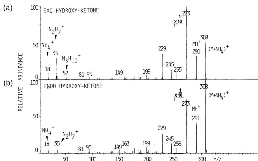
**Figure 5.** Employing the hydroxy-ketone analogs of the terpene epimers (ketone group at C-13 in place of the acetal group shown in Scheme 1), collisionally activated reaction mass spectra of  $MH^+$  ( $m/z$  291) from (a) *exo*- and (b) *endo*-hydroxyl configurations with ammonia as the reaction gas in the collision cell of the triple quadrupole.
