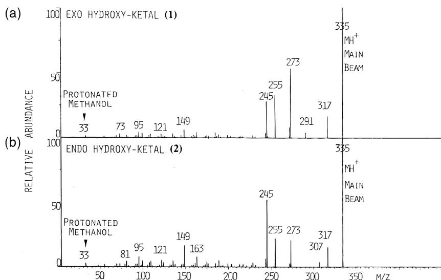
Figure 1. Collisionally activated reaction mass spectra of MH<sup>+</sup> (*m/z* 335) from (a) *exo* (**1**) and (b) *endo* (**2**) hydroxy-acetal terpene epimers with methanol as the reaction gas in the collision cell of the triple quadrupole.
