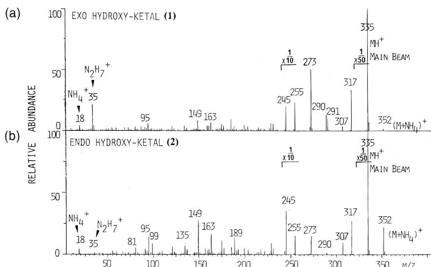
**Figure 4.** Collisionally activated reaction mass spectra of  $MH^+$  ( $m/z$  335) from (a) *exo* (1) and (b) *endo* (2) hydroxy-acetal terpene epimers with ammonia as the reaction gas in the collision cell of the triple quadrupole.
